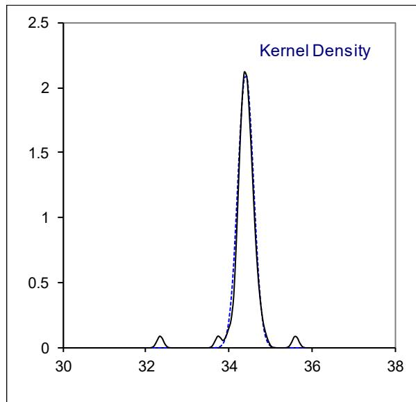
Determination of Kinematic Viscosity at 100°C on sample #19265; results in mm<sup>2</sup>/s
