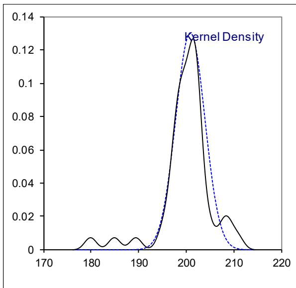
Determination of Kinematic Viscosity at 50°C on sample #19265; results in mm<sup>2</sup>/s
